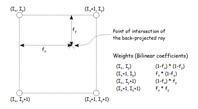
Figure 2. Local view of the reconstruction algorithm – 2x2 pixel grid and bilinear coefficients
