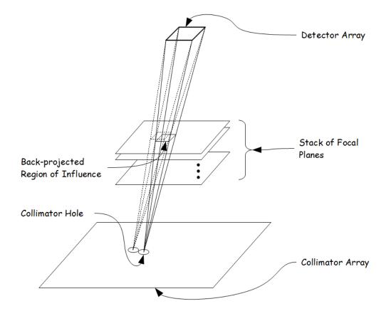
Figure 1. Basic Geometry of Tomosynthetic Image Reconstruction in the SBDX System
